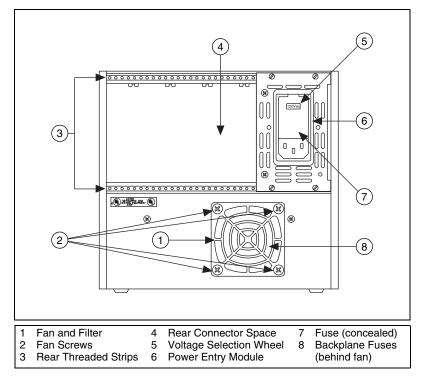
Figure 2-4. SCXI-1000 Rear View Diagram
