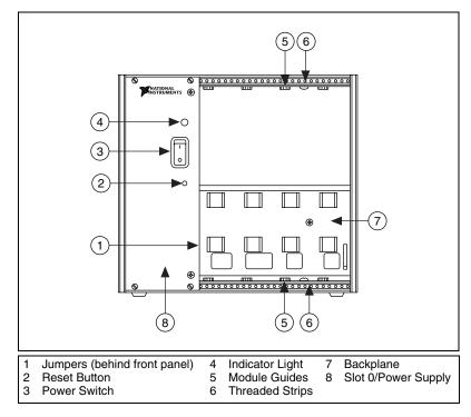
Figure 2-2. SCXI-1000DC Front View Diagram
