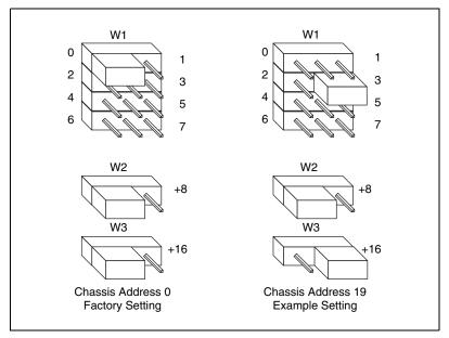
Figure 2-8. SCXI-1000DC Chassis Address Jumper Settings
