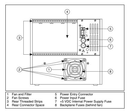
Figure 2-6. SCXI-1000DC Rear View Diagram
