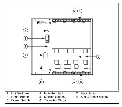
Figure 2-1. SCXI-1000 Front View Diagram
