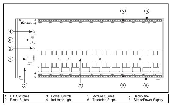
Figure 2-3. SCXI-1001 Front View Diagram
